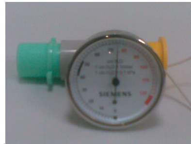
Photo-2: Showing Meter For Measuring Maximum Peak Inspiratory Pressure, i.e. (PiMax)
